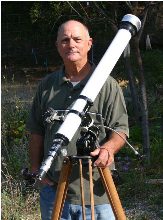
Figure 1: Grisham with his modified 1960's vintage three inch Tasco telescope on its optional tripod. Normally it is installed on a permanent steel pier imbedded in concrete. Its air-spaced objective provides remarkably sharp images.
